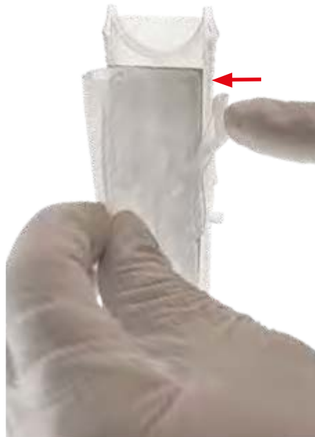
To open, press on the lever to allow the funnel to open.
