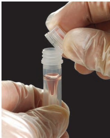
Screw Tamper Evident cap on tube until locking ring clicks over serrated tube neck.
