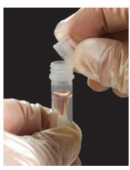
Screw Tamper Evident cap on tube until locking ring clicks over serrated tube neck.
