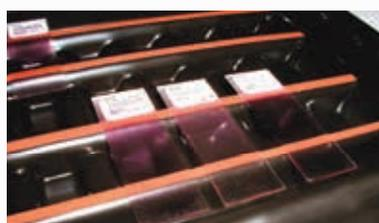
Wells between rails can be used to hold water for techniques needing a humid environment.
