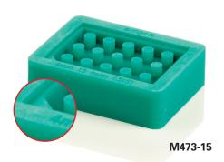
One inside wall corner at 45 degree angle, facilitating orientation.
